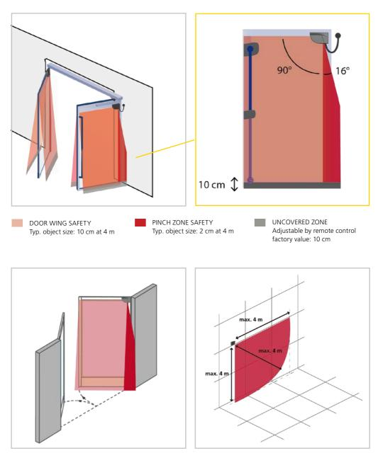
Check the detection fields using our online sizer tool: **bea-flatscan.com/sizer**
