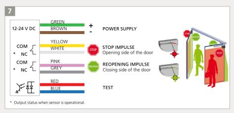
Cut the power cable to the right length, strip the 8 wires and connect all wires as indicated. The polarity of the power supply is important.
