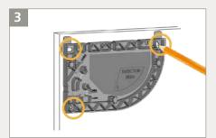
Using a pencil, mark the position of the holes to drill into the door frame. You can also use the inner surface of the base to fasten the screws.
