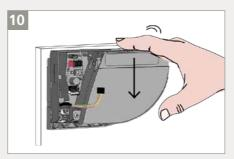
Pass the cable through the hole on the back of the sensor and fasten the sensor on the base by sliding it downwards.
