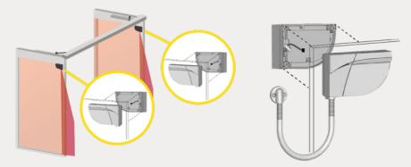
Keep a minimum distance of 15 cm between the FLATSCAN and radar sensors or use the *LZR®-FLATSCAN Protective cover* to avoid unwanted reactions of the door.
