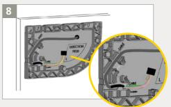
Take the master-slave cable and pass it through the hole. Position the cable in the notch of the base and make sure it is firmly fixed.
