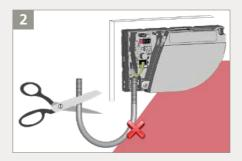
Cut the surplus to avoid undesired detections caused by the flexible tube.
