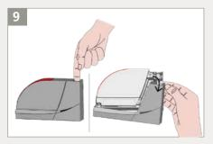
Take the sensor and remove the cover: put your finger in the hole and pull firmly towards you in one movement.
