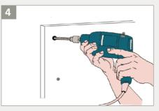
Remove the base and pre-drill the holes where marked.
