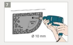
Drill through the 2 bases and the door using a 10 mm bit in order to pass the master-slave cable. Soften the edges using a sheet of sandpaper.
