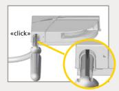
To open the sensor again, position a screwdriver in the notch and pull upwards until the cover comes loose.
