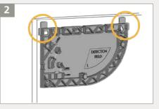
Slide the base off the sensor module.
