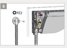
Tighten the other side of the flexible tube using the cable cap and pass through the rest of the power cable towards the door controller.
