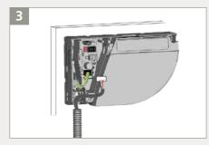
Pass the power cable through the flexible tube. Connect the white plug to the white connector.
