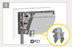
Take the clamp to fix the flexible tube to the sensor. Fasten the 2 screws firmly in order to avoid pulling out the cable.
