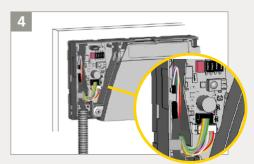
Make a loop with the wires of the power cable and pass them through the notch as indicated. Use the other part of the cable to block the wires.
