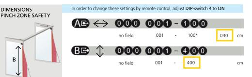
$\star$  The actual dimensions depend on the mounting height (100 cm at 4 m).
