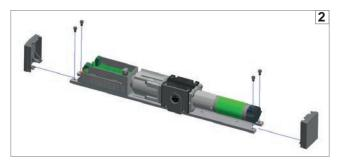
Remove the plastic side caps from the plate by loosening the socket head cap screws M5x8 (fig. 2).
