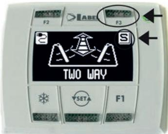
M is displayed on the top right of the display when you select the Master automation, while S is displayed when you select the Slave automation.
