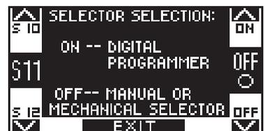
Select whether the door should only be closed by spring force (OFF), or if the motor (ON) must also be enabled to provide greater reclosing force.
