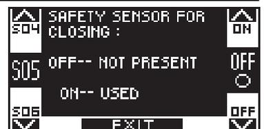
Select ON only if an opening safety sensor has been installed on E.O. input (terminal 6).
