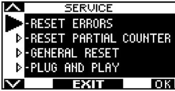
This section is accessed only to reset any fault existing in the events memory and the partial counter of the door opening/closing cycles performed by the door and to reset the initial setup carried out during commissioning. The event memory and partial counter reset must be performed by specialized personnel only during routine maintenance, after performing all system operation checks.
