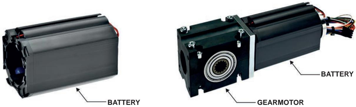
Battery supplied assembled in the plastic casing located around the motor body for the best use of the inner spaces of the automation. Plug-in connection to connect the battery to the control unit of NEXT 120S. The battery charging and monitoring circuit is incorporated in the electronic control unit of NEXT 120S. Battery life approx. 1 hour in continuous operation and 3 hours in standby.
