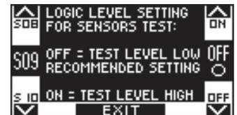
Contact configuration on OPEN input between terminals 0-3 of the control unit NEXT-L120S. Select ON with a normally open contact or when the OPEN input is not used.
