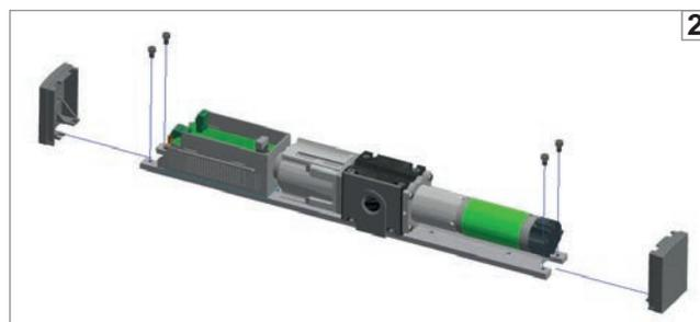
Remove the enclosure of the electronic control unit from the plate by unscrewing the two countersunk hex head screws M5x8 (fig. 3).
