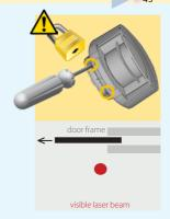
**Lock the position** of the mounting bracket to avoid malfunctioning in case of extreme vibrations.
