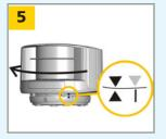
Position the housing on the bracket and turn the sensor until the two triangles are face to face.
