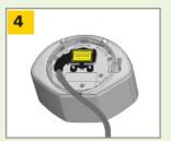
Open the protection cover, plug the connector and position the cable in the slit. Close the protection cover and fasten it firmly.
