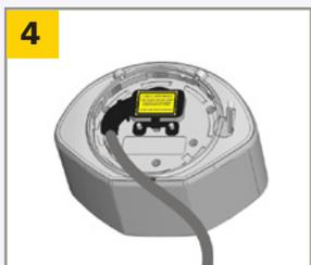
Open the protection cover, plug the connector and position the cable in the slit. Close the protection cover and fasten it firmly.
