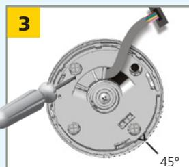
Position the bracket and fasten the 4 screws firmly in order to avoid vibrations.
