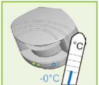
Keep the sensor permanently powered in environments where the temperature can descend below  $-10^{\circ}\text{C}$ .
