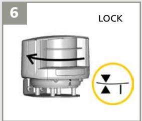
6 Turn the sensor until the two triangles are face to face.
