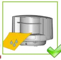
Clean the laser window with compressed air. If needed, wipe only with a soft, clean and damp microfibre cloth.
