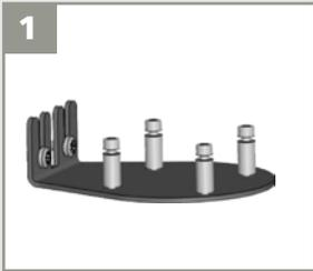
1 Use a mounting post or a mounting accessory to fix the sensor on the pole (LBA accessory for example).
