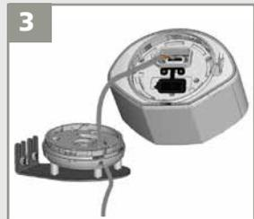
3 Open the protection cover, plug the connector and position the cable in the slit.
