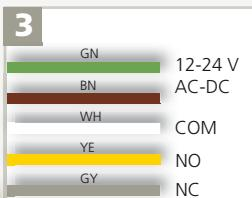
Connect the wires to the door controller. Choose between NO and NC contact.
