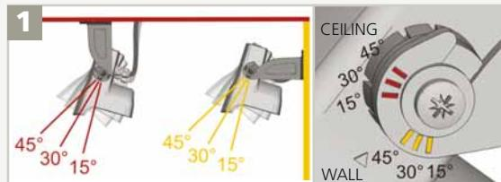
Adjust the angle of the sensor to position the detection field.
