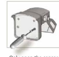
Only open the sensor when the cable needs to be replaced.
