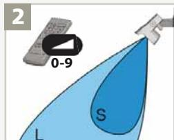
Adjust the field size with the remote control or the push buttons.
