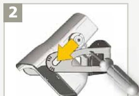
Position the sensor on the bracket and fasten the screws firmly.
