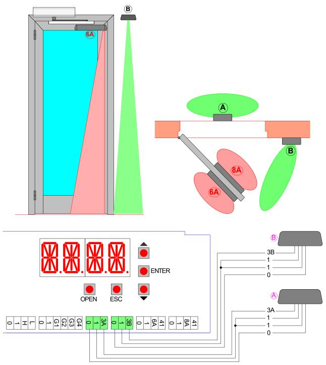
Connect the sensor, using the supplied cable to the terminals of the electronic control as follows:
