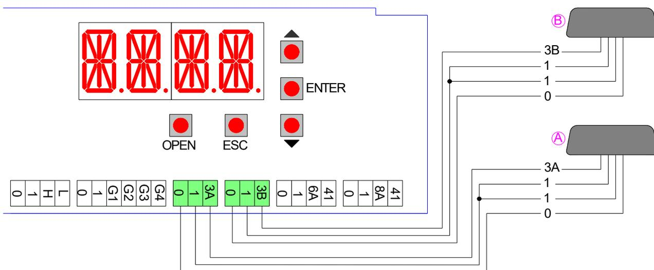
Connect the sensor, using the supplied cable to the terminals of the electronic control as follows:
