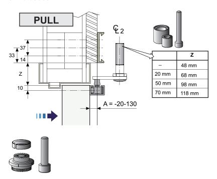
**Note!** Measurement Z must be reduced by 20 mm if lower adapter from kit 1011705BK/SI is used.
