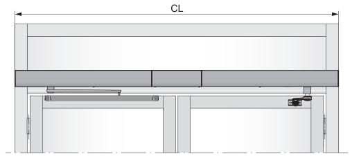
Modular cover using cover piece between two standard covers.
