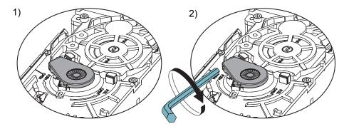
d When stop arm is on the bottom of the operator, loose the stop arm locator and the stop arm. Mount the stop arm on the splines, as close as possible to the stop block 3). Mount the stop arm locator. Fine-adjust if necessary with the screw on the stop arm 4).
