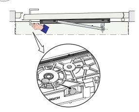
Hold the door a bit open and remove the start position pin.
