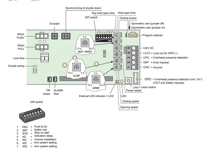
**Note!** Connect the motor cable to either PUSH or PULL depending on arm system.
