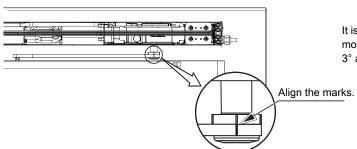
It is important to align the marks correctly. If necessary move one mark at a time. This corresponds to approx.  $3^\circ$  and will give a precision of  $\pm 1,5^\circ.$
