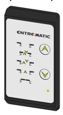
The different operation modes are selected by pushing the arrow symbols pointing upwards or downwards. When a button is pushed a buzzer will sound. The present selection is indicated by a blue light to the left of the function symbol.
