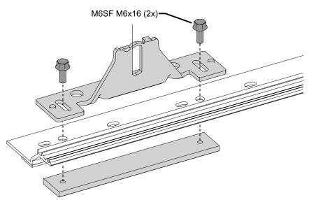
Attach the track to the bar with the screws loosely.
