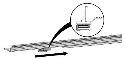
Attach the trailing door holder with screws loosely to the short bar.
