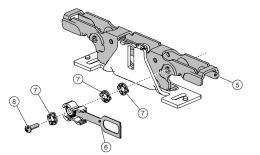
Figure 3: Maximum depth adjustment
