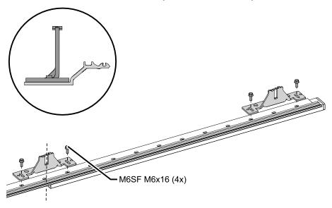
Place the L-profile and attach it with screws, placed in every other hole starting from both ends.
