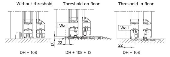
Figure 1: Installation height
