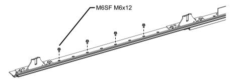
Add the plastic track and attach it with one screw in the trailing edge. Attach two screws as door stops.
