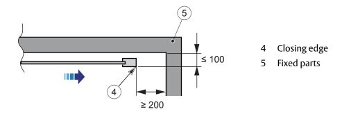
If the distance is more than 100 mm but less than 150 mm between the door and the wall the speed of the door has to be reduced acording to PRA-0004 or equip the operator with side presence sensors or pocket screens.
