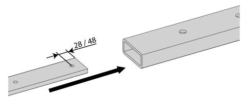
Place the secondary track on the tube with the shim inbetween. Insert the end cap.
