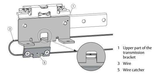
e Fasten the lower part of the transmission bracket (7) on the wheel holder (2).
