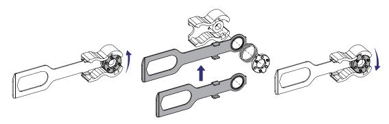
Figure 2: Switch to short spring latch
