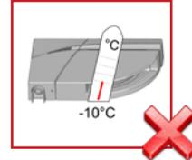
Keep the sensor permanently powered in environments where the temperature can descend below  $-10^{\circ}\text{C}$ .
