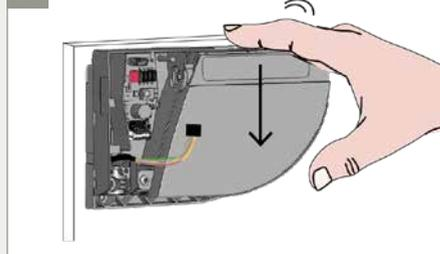
Pass the cable through the hole on the back of the sensor and fasten the sensor on the base by sliding it downwards.
