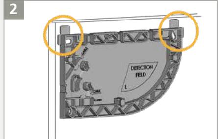
Take the base and put it on the door frame. The positioning aids help you to align the base correctly.
