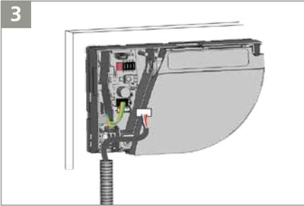
Pass the power cable through the flexible tube.
