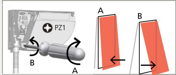
If necessary, adjust the tilt angle of the laser curtain by turning the tilt angle adjustment screw (from 2° to 10°).
