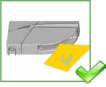
Clean the laser window with compressed air. If needed, wipe only with a soft, clean and damp microfiber cloth.
