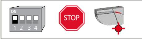
RELAY 1: STOP-impuls on the opening side of the door
