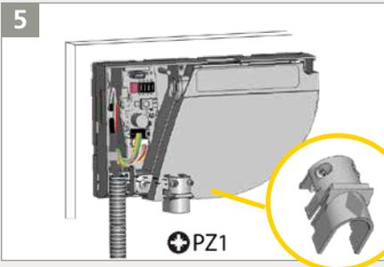
Take the clamp to fix the flexible tube to the sensor.
