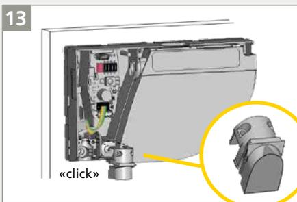
Close the sensor which will not be connected to the door controller using a plug.
