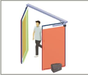
Check the correct positioning of the safety fields by placing an object in the detection field.
