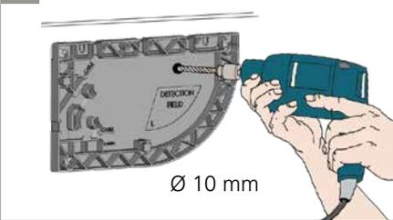
Drill through the 2 bases and the door using a 10 mm bit in order to pass the master-slave cable. Soften the edges using a sheet of sandpaper.
