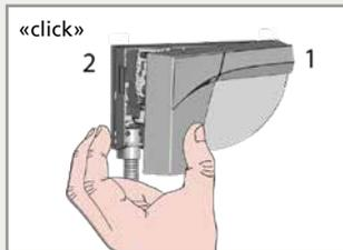
Close the cover starting on the narrow side (1). Do not hesitate to push.
