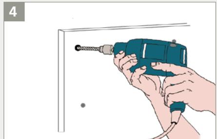
Remove the base and pre-drill the holes where marked.
