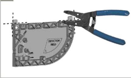
Using a wire cutter, remove the positioning aids from the base.
