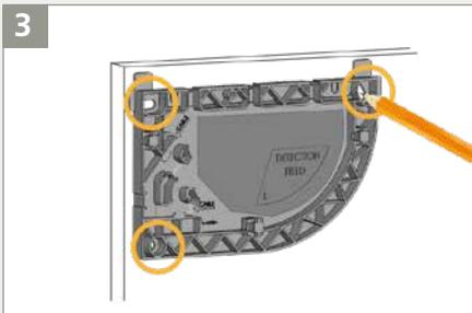
Using a pencil, mark the position of the holes to drill into the door frame. You can also use the inner surface of the base to fasten the screws.
