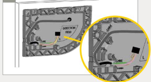
Take the master-slave cable and pass it through the hole. Position the cable in the notch of the base and make sure it is firmly fixed.
