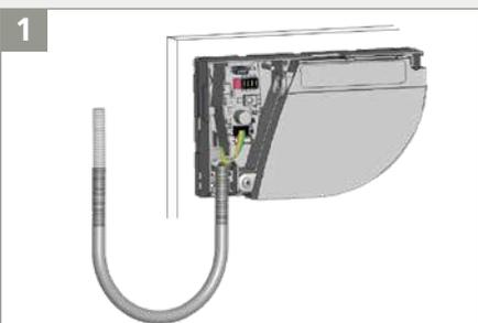
Take the flexible tube and determine how long it should be in order to reach the door controller.
