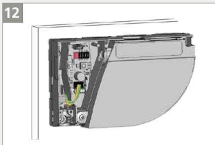
Make sure that all wires are safely tucked within the notch to avoid crushing them with the cover.
