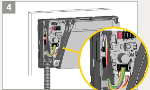
Make a loop with the wires of the power cable and pass them through the notch as indicated.
