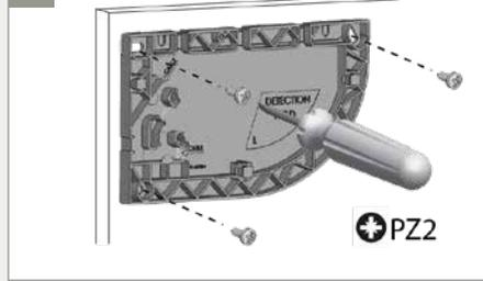
⚠ Fasten the 3 screws using a Pozidrive screwdriver. The base needs to be fixed firmly!
