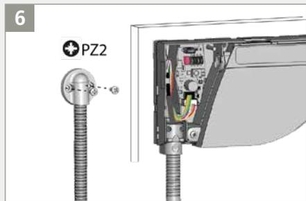
Tighten the other side of the flexible tube using the cable cap and pass through the rest of the power cable towards the door controller.
